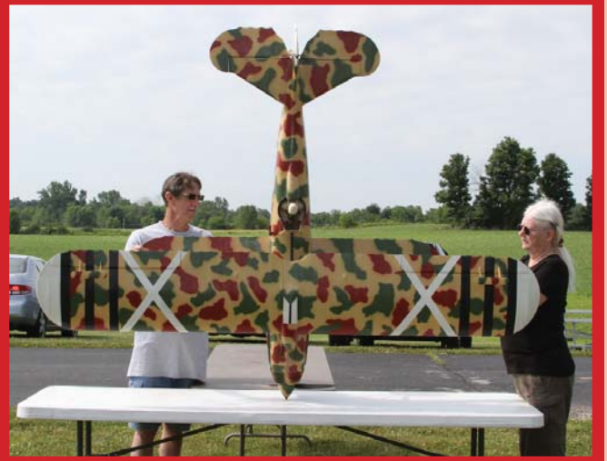
Larry Botsford and his wife hold their Fiat CR.32, which was entered in the Designer Class, for the static judges. It was scratch-built from Larry's own plans and is covered in Solortex.
