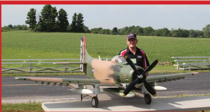
Lawrence Harville holds his entry in Expert class, a Nick Zirola Douglas Skyraider with a 101-inch wingspan. It's powered by a DLE .61 gas engine, is painted with Behr Latex paint, and has 12 droppable rockets, two droppable napalm tanks, and one center tank.
