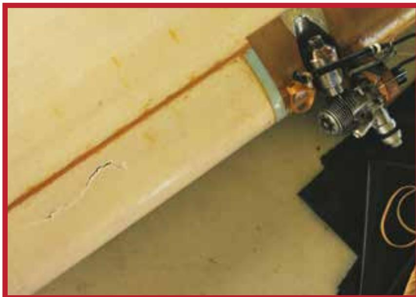
It will probably be hard to see, but from the leading edge back toward the spar, there is a fine line showing where the string cut through the foam, ending in a triangular dent. The open crack in the foam is where the impact broke the hollow foam leading edge, letting the knot slip through. If the string had cut all the way back to the spar, the knot probably would have caught there and broken the string.
