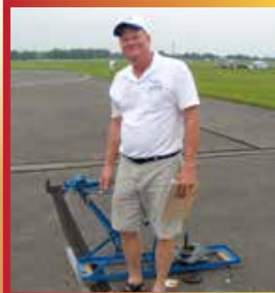
Don Main mans the pull test device between circles 1 and 2.
