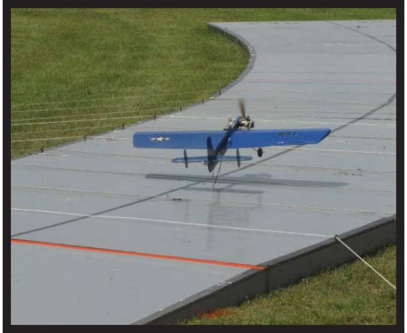
Landing can be a challenge when the touchdown area is only 20 feet long. The tailhook engages one of the arresting cables, bringing the model to an abrupt halt. This is Paul Kegel's Grumman Guardian about to make a perfect arrested landing.
