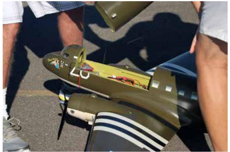
The forward section of the DC-3 fuselage comes off to allow for the batteries to be installed and service the model.
